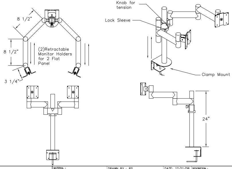
NOTES: DRAWN BY: RS DATE: 12/11/06 DESCRIPTION: AS NOTED ABOVE MONITOR ARM-CLAMPED POLE MOUNT R O V Α E D TOLERANCES UNLESS OTHERWISE SPECIFIED USED ON: ENG: MFG: FRACTIONAL 2 PLC. DEC. 3PLC. DEC. ANGULAR ±.01 ACCESSORIES\MONITOR ARMS\Z SERIES/2006 ±.5° QA: PDF NAME: AFCZ200-02 SHEET: 1 OF 1 **FINISH** SCALE: N.T.S.
